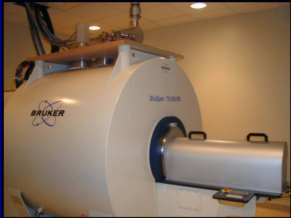
Biospec MRI 7 Tesla, 30 cm bore
